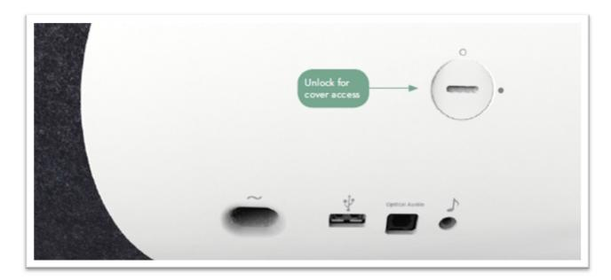
Remove power cable, stand and the 2 screws on the backside of the speaker. Once the backplate is removed - unzip the wool cover.
