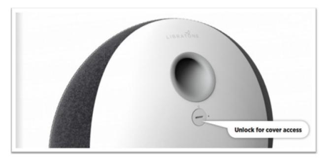
Remove power cable, stand and the screw on the backside of the speaker. Once backplate is removed - remove the wool cover.
